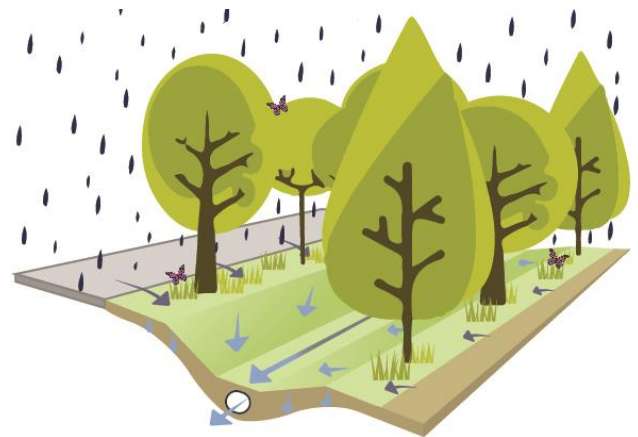
Diagram of a nature-based solution (swale) in action
